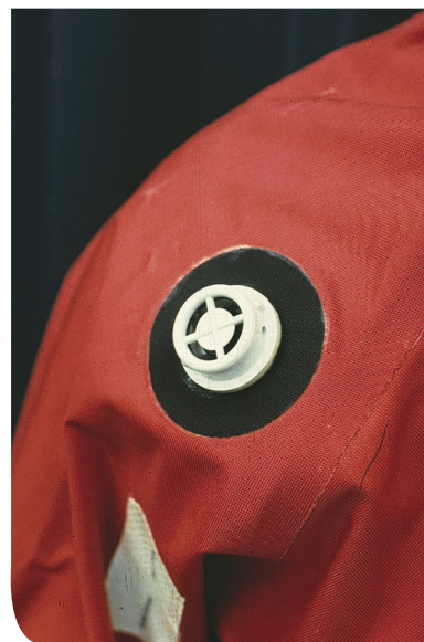
Figure 24: An example of a relief valve fitted on the crest of the shoulder. In this case, a valve is also fitted on the other shoulder and in some cases, valves are fitted in the feet too.
