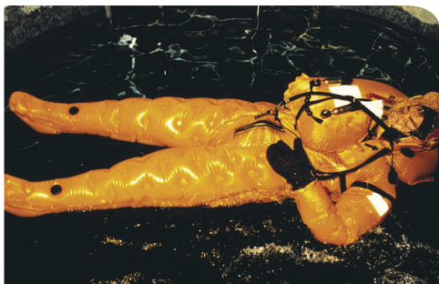
Figure 40: The Shell, Shark Group, University of Surrey RF heat sealed inflatable survival suit worn with an asymmetric lifejacket to ensure self-righting.
